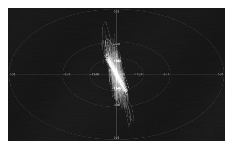
A Lissajous is essentially an oscilloscope where a secondary signal drives the X-co-ordinate of the oscilloscope trace. It can be used to visualise stereo width of a signal, as it forms a balance between stereo image display and a more general-purpose oscilloscope.
