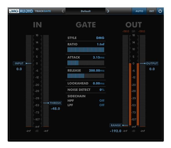
TrackGate is a fully-featured noise gate, expander, ducker and MIDI gate. A good gate can make the difference between re-recording and a great mix.
