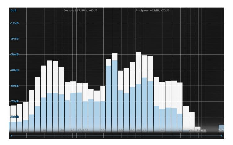
The 1/N Octave analyser is a reformatting of the data from the FFT Analyser into octave, 1/3rd octave or 1/12th octave bands. It is not an RMS analyser (described below), but is extremely convenient for quick analysis.
