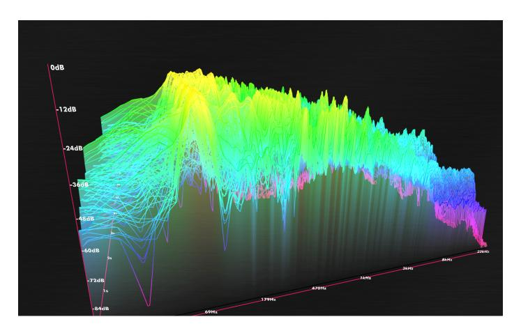
The 3D Spectrograph is a three-dimensional rendering of the 2D Spectrograph, which allows for a surprising amount of insight into the spectral and temporal makeup of a signal. It renders a single mono signal.
