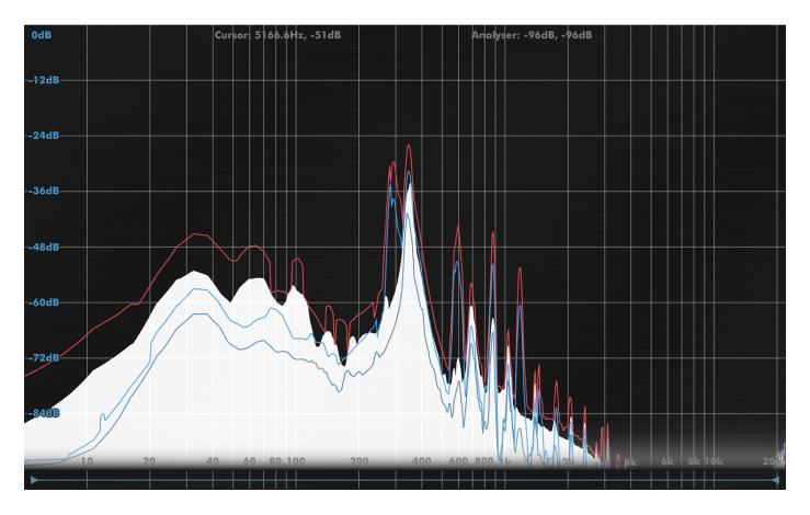
The FFT Analyser shows you the instantaneous spectral makeup of your signal. It can display two channels of information simultaneously, alongside peak information.
