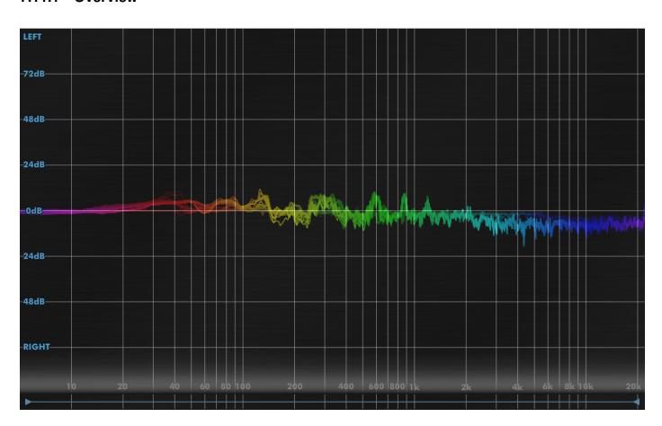
The Phase Spectrum renders the instantaneous difference in stereo position by frequency.
