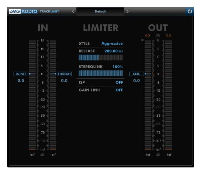
TrackLimit is a very low-latency wideband limiter, integrating the adaptive dual-stage mechanism from our flagship Limitless.
