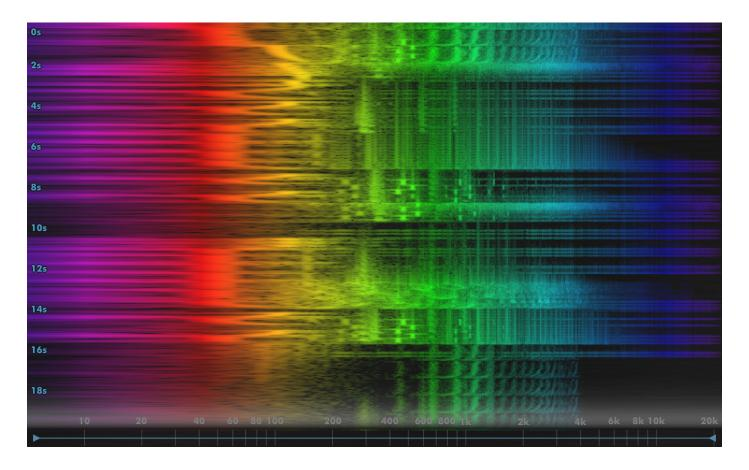
The spectrograph shows a scrolling display of frequency information over time. It can be configured to visualise individual notes, or to view broader balance of audio.
