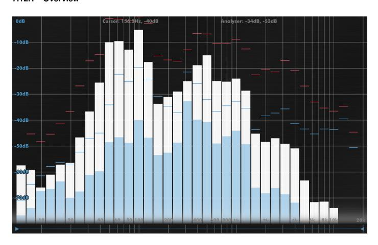
The RMS Analyser is a classic 1/3rd octave analyser design based on overlapping 36dB/oct Butterworth Band-pass filters, with per-band peak detection. This has the advantage of even
