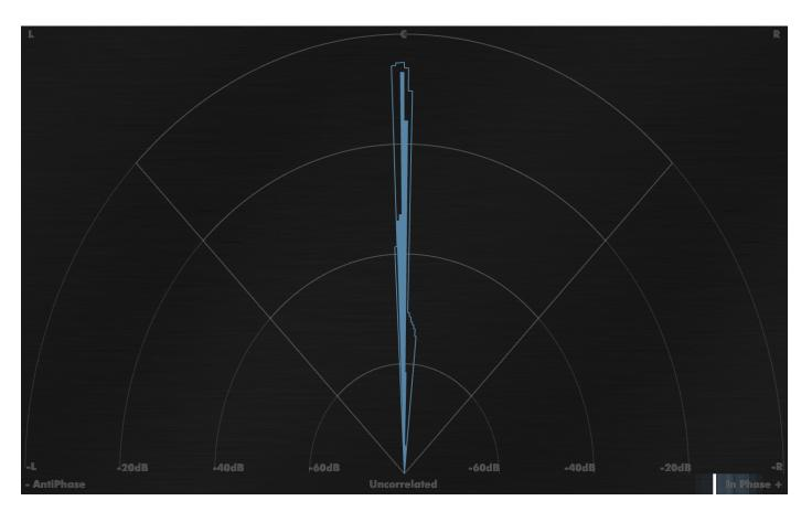
The Phase Meter provides a map of the stereo field, so you can watch stereo movement of elements in a signal. The display renders directly up as mono, hard left and hard right at 45 degree offsets, and anti-phase data to the extremes. It requires a stereo signal source.
